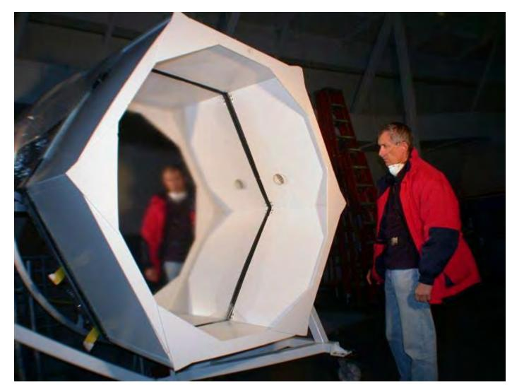
Spray Application of First Contact Polymer to Keck 6ft hexagonal mirror.
