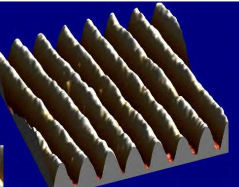
False color images obtained after applying a fingerprint to the 300nm grating, applying polymer & removing the film after allowing it to dry. Notice preexisting defect at left. Some of these gratings were "seconds" from the manufacture.
