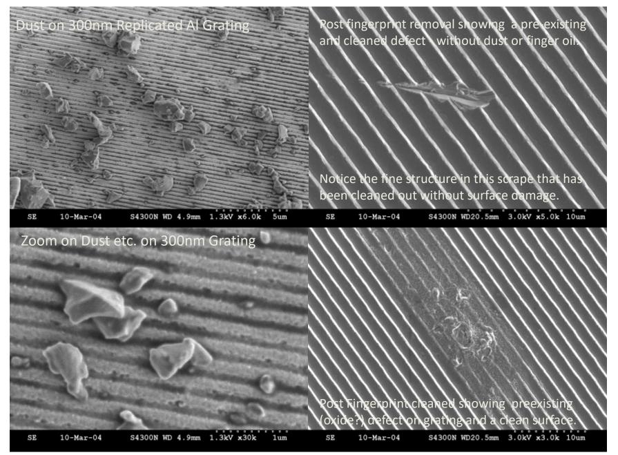
Precleaning and Post Fingerprinting, Cleaned Surface on Hitachi S-4300 Cold FE-SEM
