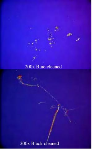
First Contact Polymer: Completely Clean using Nomarksi Interference Microscopy
