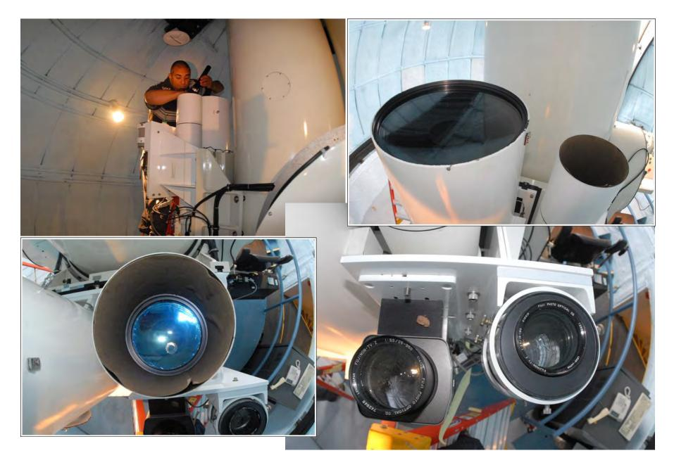
Applying a protective coating of the *First Contact* Polymer to the Visible Wavelength Dahl-Kirkham Telescope
