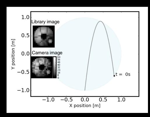
Guiding on an 8<sup>th</sup> magnitude, solartype star. Trajectory fire occurs at 0s. Pupil plane camera exposure time is 1 second. Precision is 2 cm.
