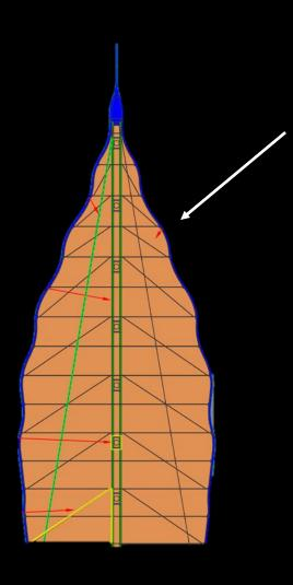
To avoid solar glare and scatter interference petal optical edges must be razor-sharp <u>and</u> exceedingly clean
