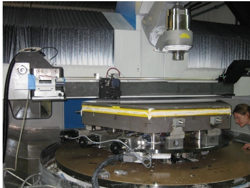
On-machine deployment of pentaprism profilometer
