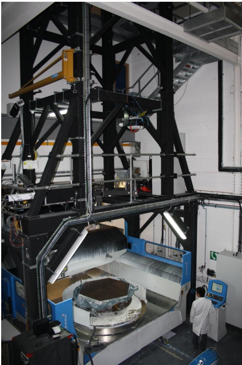
Zeeko IRP1600 under test-tower On-axis optical test
