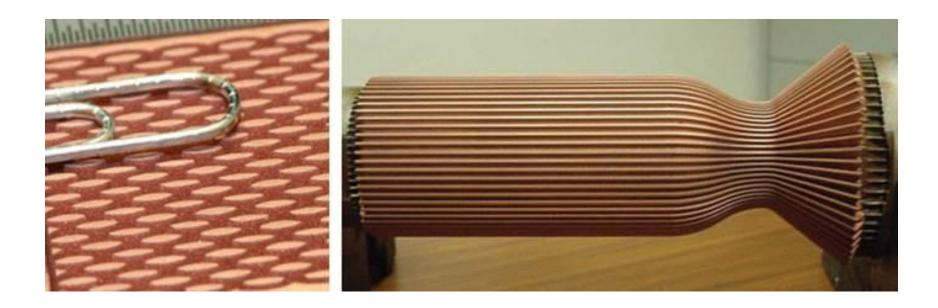
2015 phase II SBIR: Low Cost Manufacture of nozzles and combustors for channel wall liquid rocket engines.
