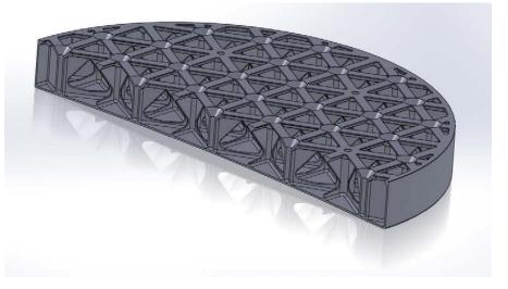
Wall thickness: 0.89mm Diameter 0.24 meter Thickness: 25.4 mm Spherical Mirror - 2.3 meter radius Weight: 0.483 kg Areal density: 10.6 kg/sq meter Wall thickness: 0.51mm Diameter 0.24 meter Thickness: 25.4 mm Spherical Mirror - 2.3 meter radius Weight: 0.28 kg Areal density: 6 kg/sq meter
