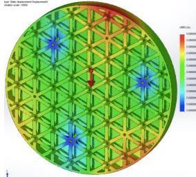
Internal bracing allows tailored stiffness to make the rear Mounting surface of the mirror Substrate stiffer than the front optical contoured surface.
