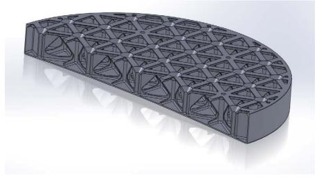
Wall thickness: 0.89mm Diameter 0.24 meter Thickness: 25.4 mm Spherical Mirror - 2.3 meter radius Weight: 1.4 kg Areal density: 31 kg/sq meter Wall thickness: 0.51mm Diameter 0.24 meter Thickness: 25.4 mm Spherical Mirror - 2.3 meter radius Weight: 0.8 kg Areal density: 17.6 kg/sq meter
