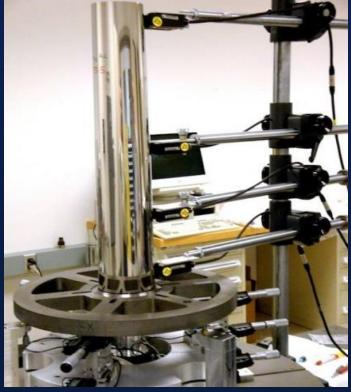
The x-ray optics module alignment station used for the FOXSI project
