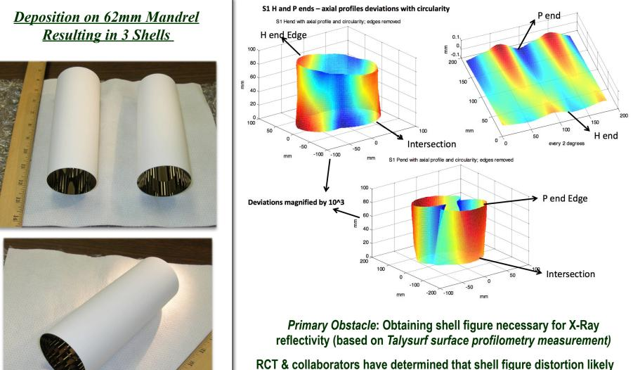
RCT & collaborators have determined that shell figure distortion likely derives from relatively high internal stresses during thermal spray coating deposition
