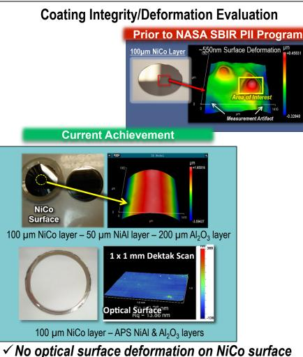
No optical surface deformation on NiCo surface
