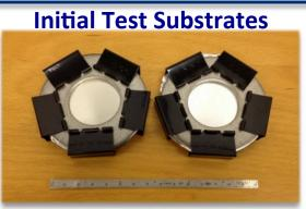
Evaluate potential particle damage using nickel and aluminum foil
