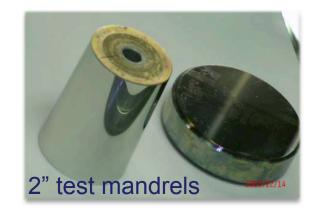
Process development using NiCo plated silicon wafers (due to mandrel availability), continued testing on conical mandrels to evaluate X-ray performance
