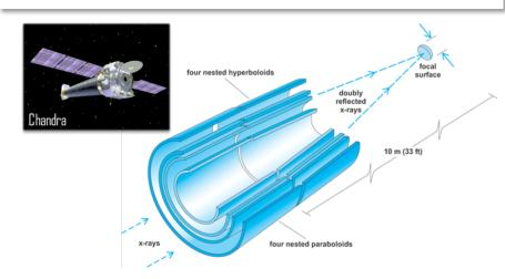
Chandra X-ray observatory utilizing 4 nested zerodur optics with the outer shell measuring 1.2 meters in diameter.
