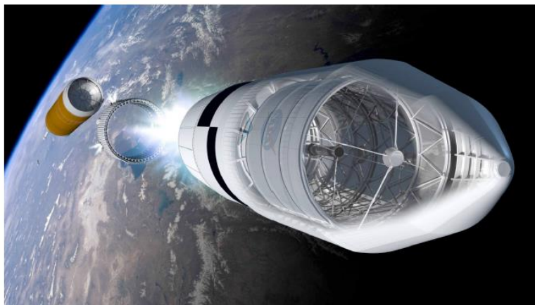
Cut-away (and simulated) view of an Ares V launch vehicle containing the ATLAST-8m payload
