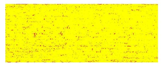
Porosity (shown in red) of cross section of DSS-19 after infusion trials. Porosity is at 2.09%
