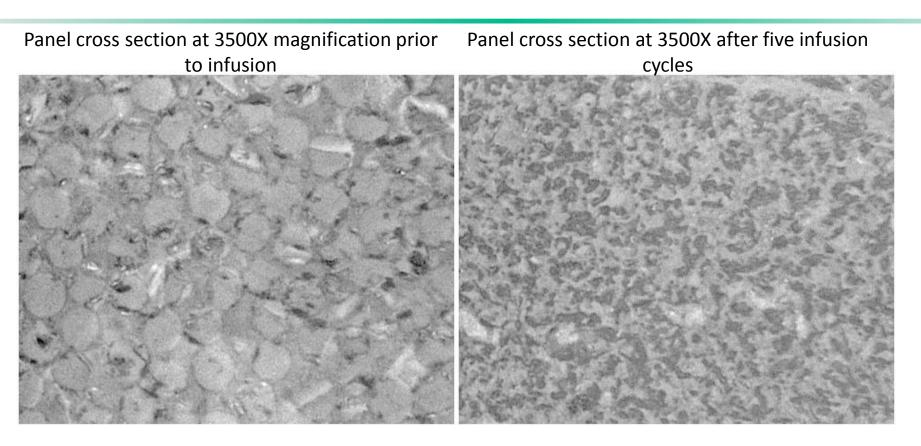
Note that the individual quartz fibers are still round and have definition on the left. After the infusion process, the fibers have lost their round shape and definition, indicating that conversion is happening
