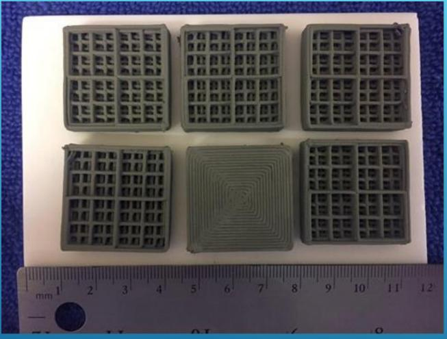
As-Printed and Cured. Feature sizes <0.8mm Also demonstrated joining in "green-state"
