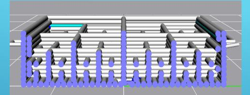
Gradient Lattice Structure: 100% dense facesheet (bottom layer) to ~27% dense, 11 total layers. Reverse Pattern to Close-Out Backside for Highest First Mode and Dimensional Stability (like a SLMS)
