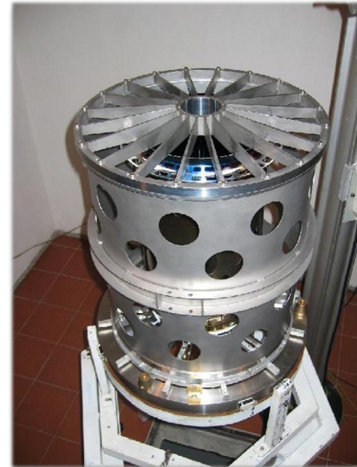
Prototype Multilayer Coated Electroformed Hard X-ray Telescope (NASA/MSFC and Brera Obs.)
