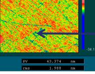
The grain boundary is visible, but not pronounced.
