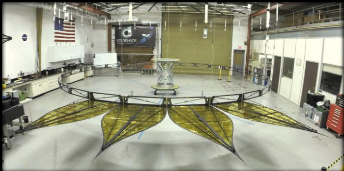
Half-scale inner disk testbed (JPL)
