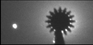
Suppressing scattered light off petal edges from off-axis Sunlight
