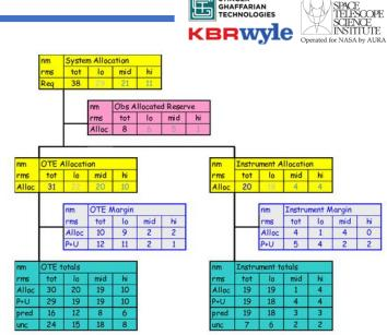
Top Level Wavefront Error Budget for LUVOIR in picometers RMS as a function of spatial frequency.
