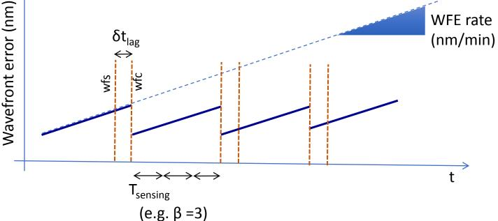
**Total sensing time follows a fundamental** property: T<sub>sensing</sub> x N<sub>phot</sub> x Contrast >1
