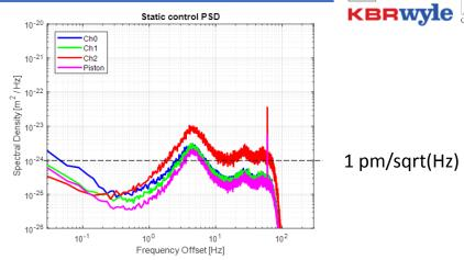
Measured Closed Loop Performance of Ball Capacitive Edge Sensor (2018)
