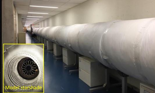
S5's starshade model validation testbed at Princeton.
