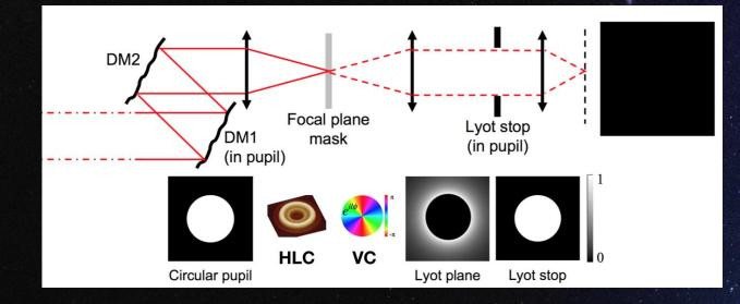
The ExEP Decadal Studies Testbed (DST) strives to achieve 10<sup>-10</sup> raw contrast for an unobscured aperture.
