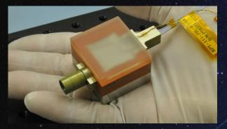
PLC beam launcher
