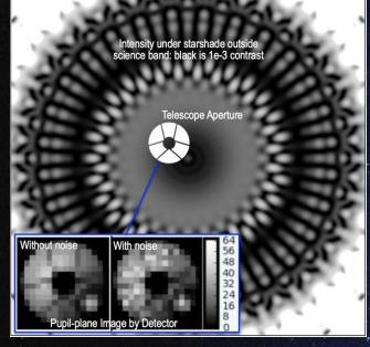
Illustration of lateral sensing using pupil-plane image matching
