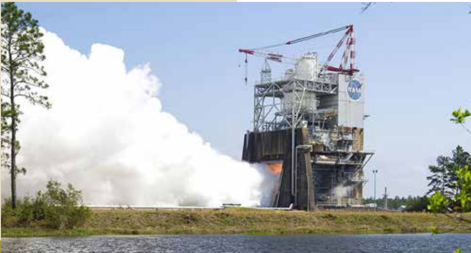
NASA engineers conduct a test of the first RS-25 engine controller that will be used on an actual Space Launch System flight on the A-2 Test Stand at Stennis Space Center on March 23. The RS-25 engine, with the flight controller, was test fired for a full-duration 500 seconds.
